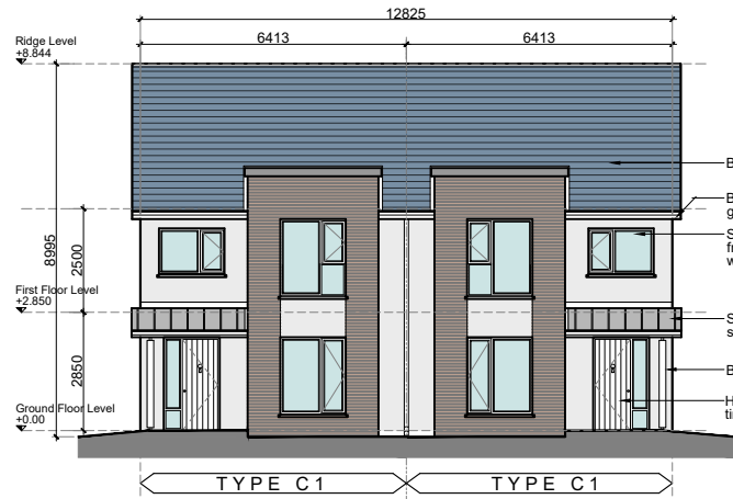
Front Elevation - Scale 1:200 Block Type C1 - Option 3
