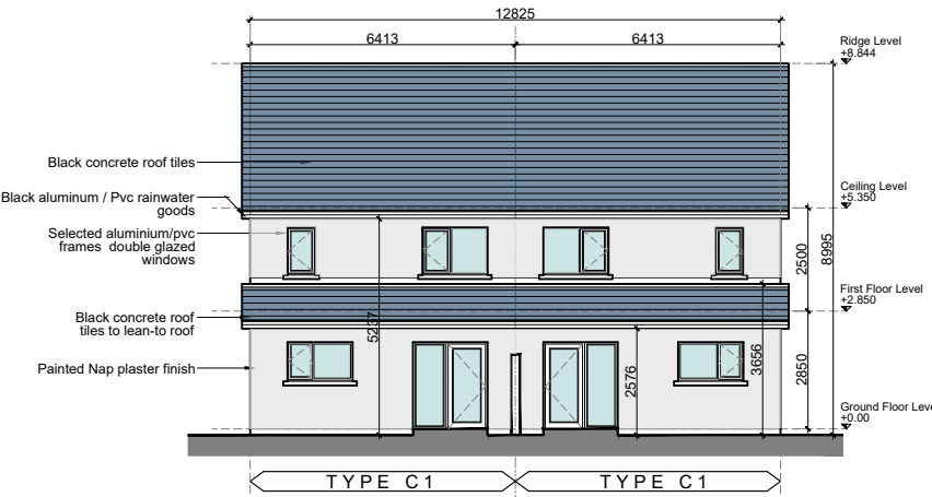
Rear Elevation - Scale 1:200 Block Type C1 - Option 3
